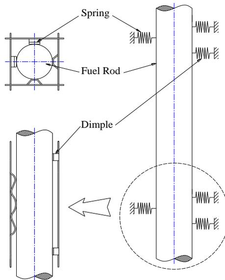
Figure 3: FE Model of CNPP Fuel Rod
