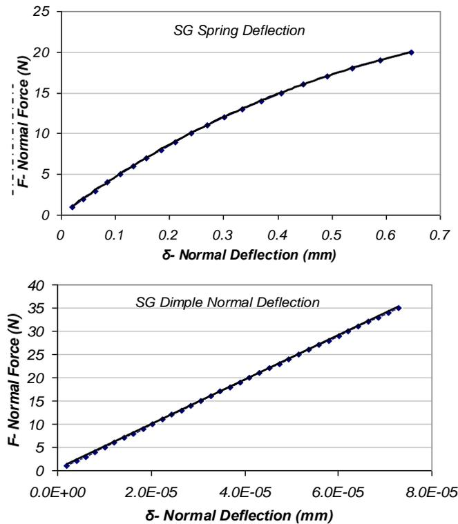
Figure 5: SG Spring & Dimple Deflection Curves
