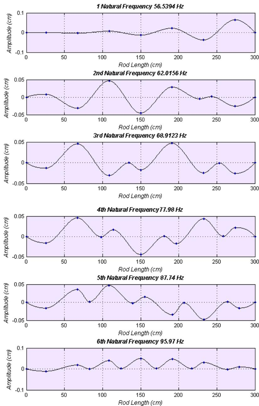
Figure 6: Mode Shape of CNPP Fuel Rod
