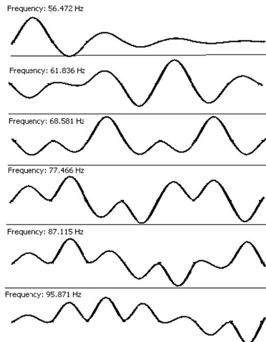
Figure 9: Fuel Rod Mode Shape using ANSYS
